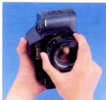
Dismounting Press the lens release button and rotate the lens counterclockwise 1/5th turn.
