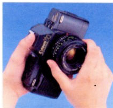
Mounting, step 2 Rotate the lens clockwise 1/5th turn until the click sound is heard
